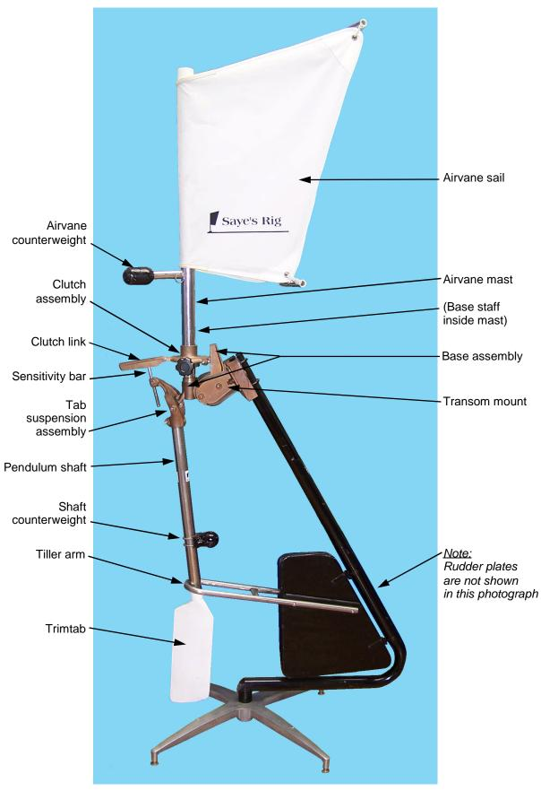
Saye's Rig on display stand (Pendulum shaft and tiller bar are necessarily shortened)
